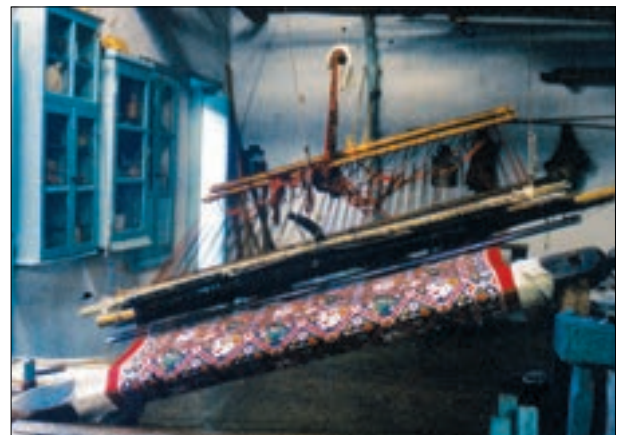
Figure 6. A view of the loom. Finished cloth is visible on the breast beam.
