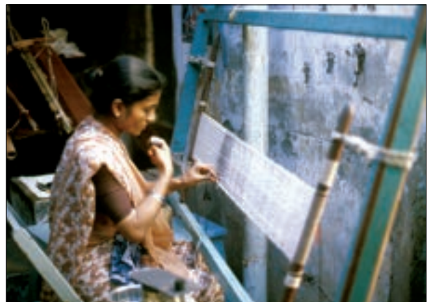
Figure 3. Tying weft bundles to match the warp.
