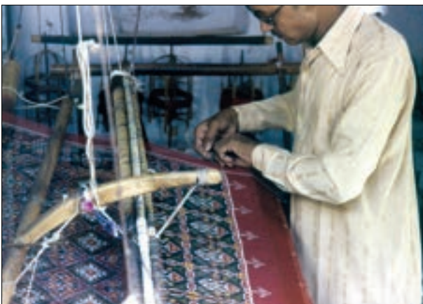
Figure 5. Setting up the warp on the loom. Notice that the pattern is visible even though the fabric is not woven yet.
